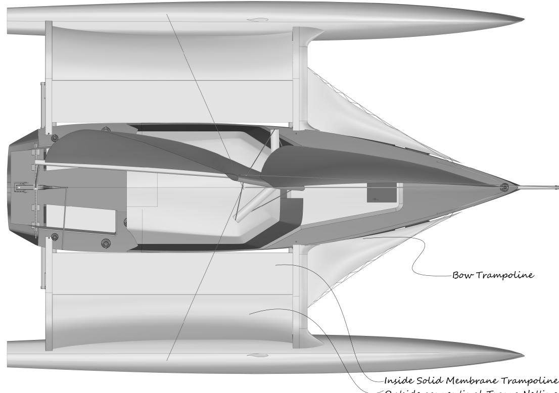
Inside Solid Membrane Trampoline Outside conventinal Tramp Netting So no time consuming need to undo
